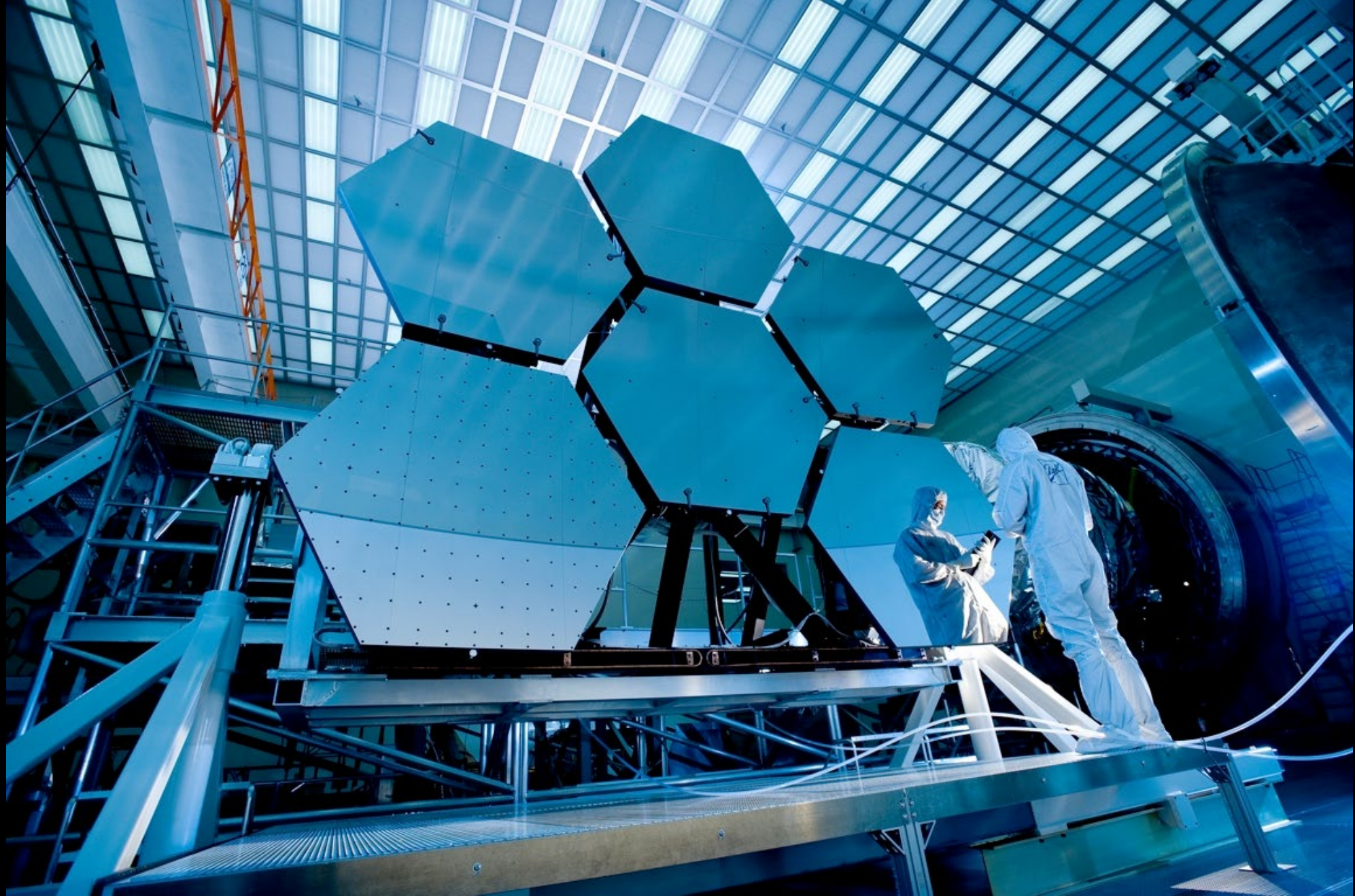
The 18 mirror segments being manufactured
