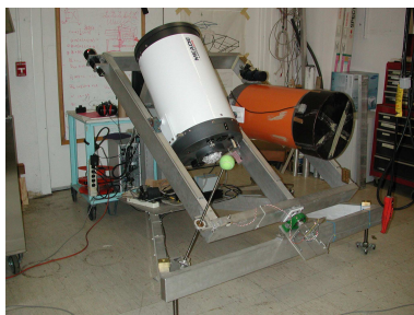
FIG. 4: Celestron 14 inch aperture, f/11 and MEADE (16 inch aperture, f/11, on aluminum mount designed to hold up to six telescopes)
